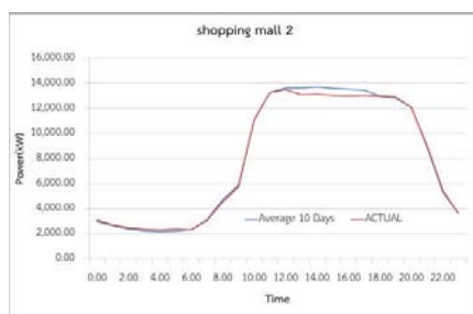
Figure 3. The power reduction from DR tested of the shopping mall 2
