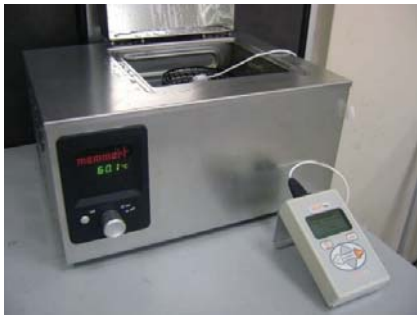
Figure 1. Thermal Conductivity measurement setup using thermal constant analyzer technique
