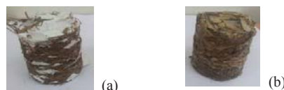
Figure 1. (a) Unused plastic RDF and (b) used plastic RDF
